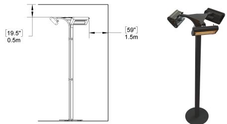
NOTE: DO NOT POINT HEATER DIRECTLY AT SIDE WALL. MINIMUM 6' FRONTAL CLEARANCE TO FLAMMABLE OBJECTS.
